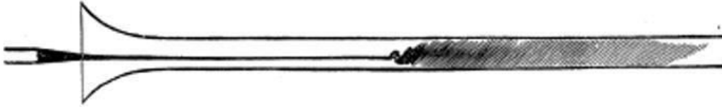
Fig. 3 The flow of dye forming wavy pattern at medium velocity
