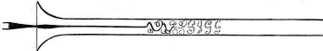
Fig. 4 The flow of dye is complex at higher velocity
