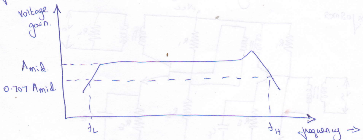
fig. Frequency response of transformer coupled amplifier.
